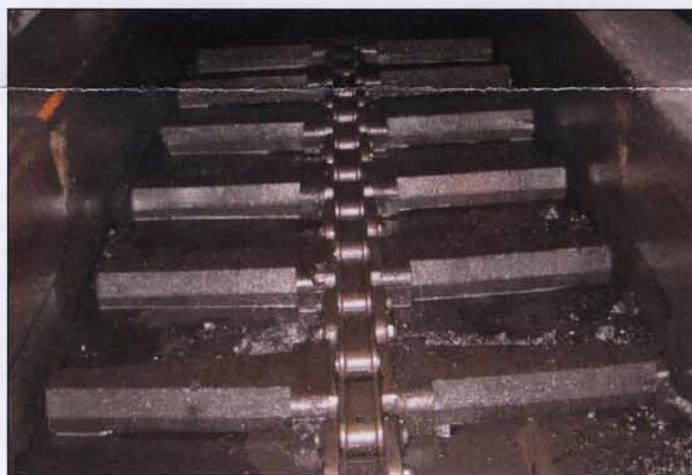
Figure 1.—Urethane-coated flight bar chain used in the conveyor system for a continuous mining machine.
