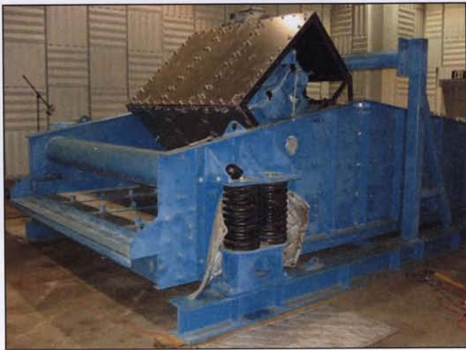
Figure 2.—Panels can be easily removed for mechanism housing maintenance.
