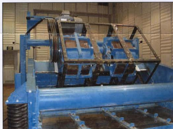
Figure 1.—Steel frame for the acoustic enclosure installed on a Conn-Weld G-Master 1000 vibrating screen.
